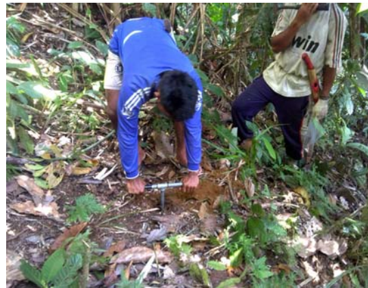
② Sampling from B Layer by Auger
