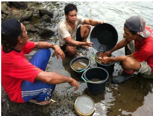
③ Sieving 2 – Collecting samples by using a 80mesh(0.177mm) sieve
