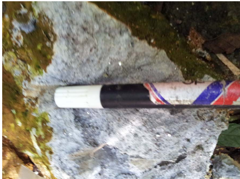
Photo 7-19 Disseminated Pyrite within Altered Andesite
