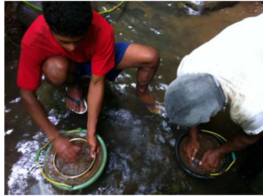
② Sieving 1 – Collecting a 20ℓ uniform sample by using a 10mesh(2.0mm) sieve
